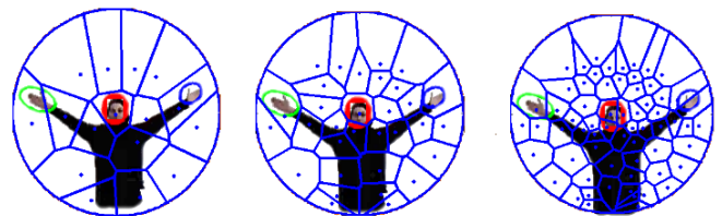
Fig. 4. Results of the Linde-Buzo-Gray vector quantization method used to split the normalized feature space into 16, 32 and 64 sectors that can be used to transform the continuous features into discrete symbols
